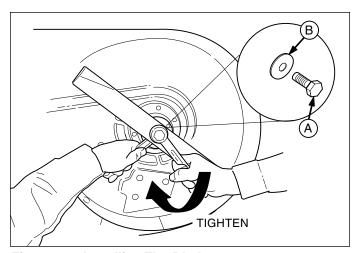
Figure 28. Installing The Blade
